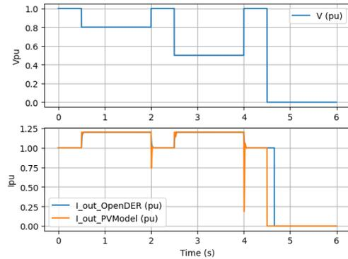
Fig. 5. Comparison of OpenDSS Dynamic PV Model to OpenDER Model
