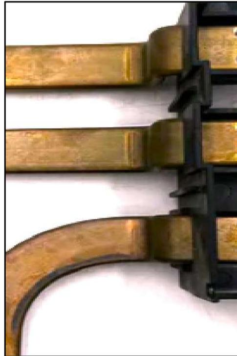
Fig. 13. New bus bars for comparison for a 1200 A CB cabinet.
