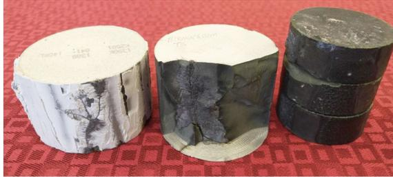
a) Tracking due to moisture. b) Puncture due to excessive energy. c) Surface melting due to flashover
