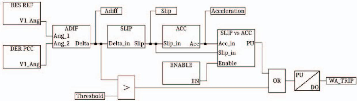
Fig. 10. RTAC Synchrophasor-Based Islanding Detection Logic
