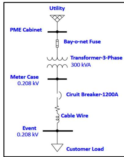
Fig. 8. One-line from the utility to an arc flash event.
