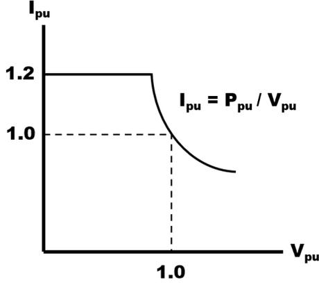
Fig. 2. Simple PV Model I-V Relationship
