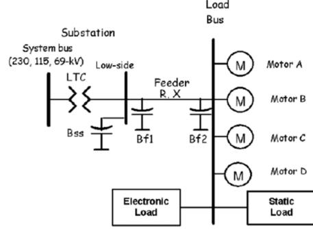
Fig. 3. Original Composite Load Model [17]
