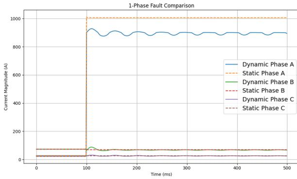
Fig. 9. Single Phase Fault Current Comparison for 25% BTM PV Penetration
