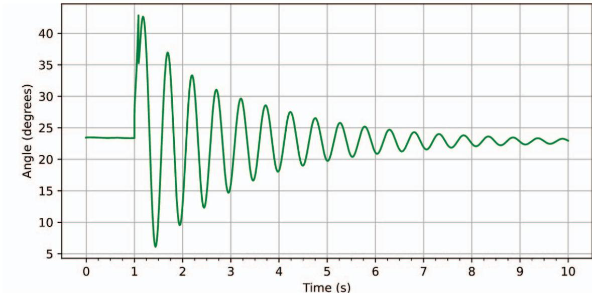
Fig. 18. Voltage Angle Difference Between Switchyard D West Bus and Substation E During a Fault at Substation B with All Units in Service (Winter)
