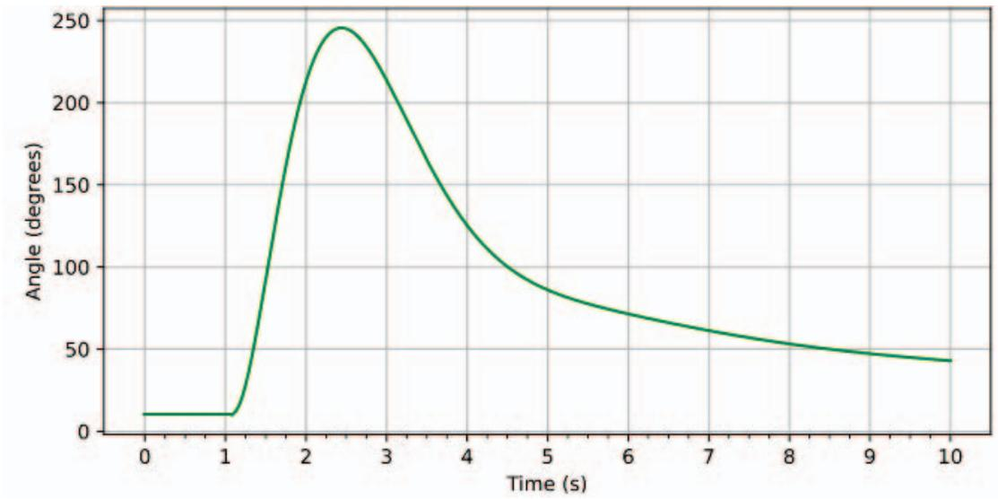
Fig. 12. Voltage Angle Difference Between Switchyard D East Bus and Substation E During an Island at Substation B 115 kV Bus with 2 Units in Service
