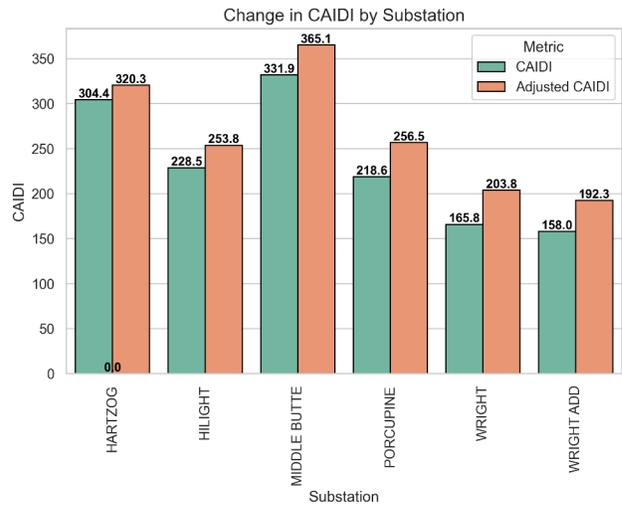
Fig. 4. Adjustments to CAIDI when factoring in added response time from PRECorp’s Gillette shop.
