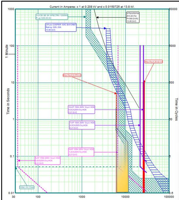
Fig. 10. TCC for probabilistic gradient for a first-degree burn after the 1200A breaker.
