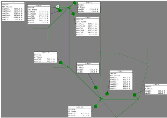
IMAGE 4: Arc flash calculations using the 12 MVA transformer.
