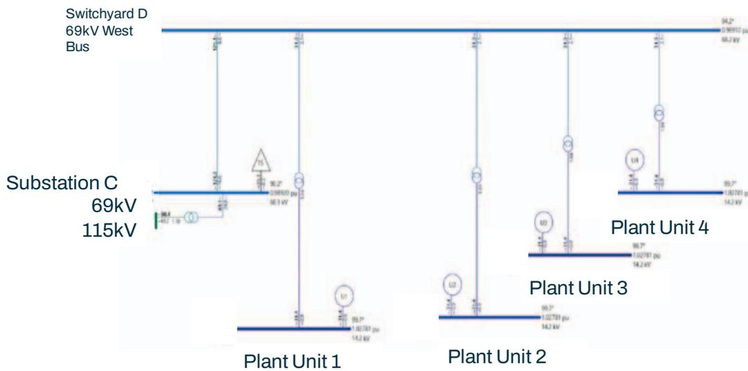
Fig. 2. WECC 2025 Light Winter Model of Switchyard D – Loop C – West Bus
