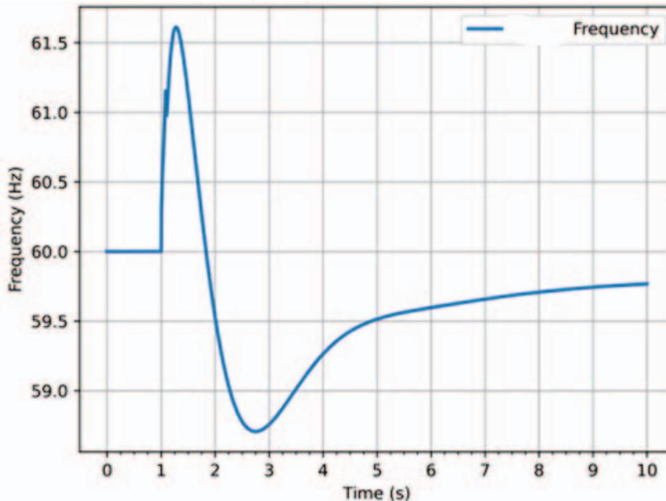
Fig. 7. Switchyard D West Bus Frequency for Island at Substation C T3 with 1 Unit Online (Winter)
