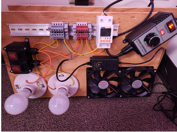
Fig. 1. Smart Circuit Breaker Demonstration Board
