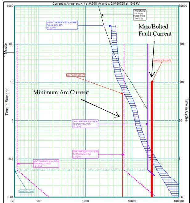
Fig. 5. Addition to Figure 4 the max fault and arcing current levels.
