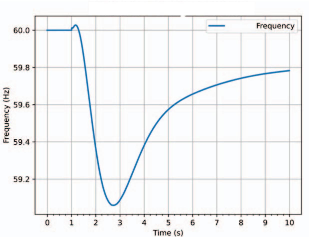
Fig. 8. Switchyard D West Bus Frequency for Island at Substation C T3 with 1 Unit Online (Winter) (Operator Error)
