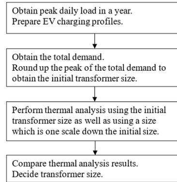
Fig. 1. Transformer sizing procedure
