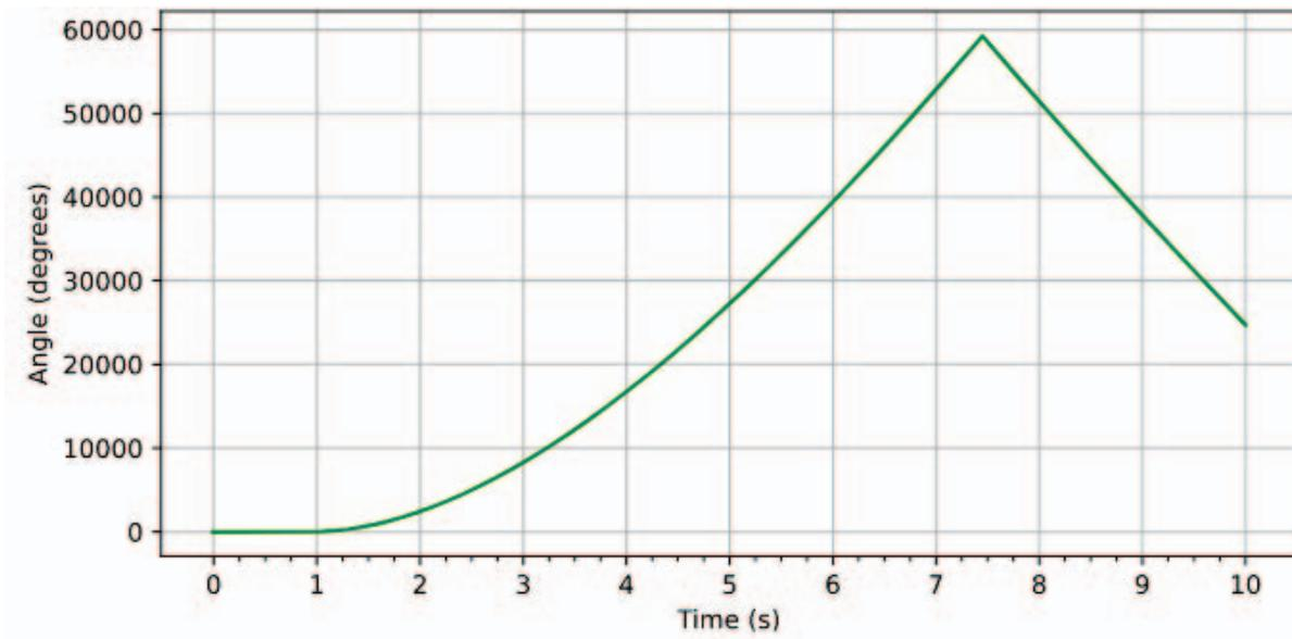
Fig. 16. Voltage Angle Difference Between Switchyard D East Bus and Substation E During a Fault at Substation B with All Units in Service (Winter)
