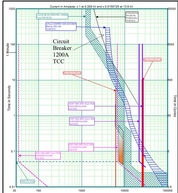
Fig. 9. TCC for probabilistic gradient for a second-degree burn after the 1200A breaker.
