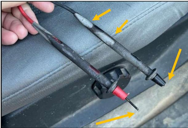
Fig. 11. Damaged meter leads.
