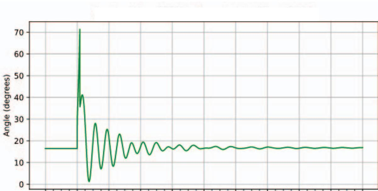
Fig. 14. Voltage Angle Difference Between Switchyard D East Bus and Substation E During a Fault at Substation B T1 with 2 Units in Service
