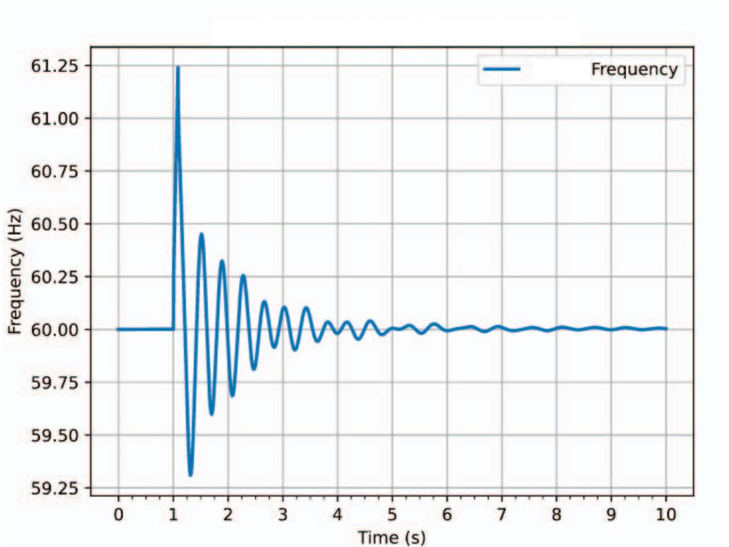
Fig. 13. Switchyard D East Bus Frequency for Fault at Substation B T1 with 2 Units Online (Summer)
