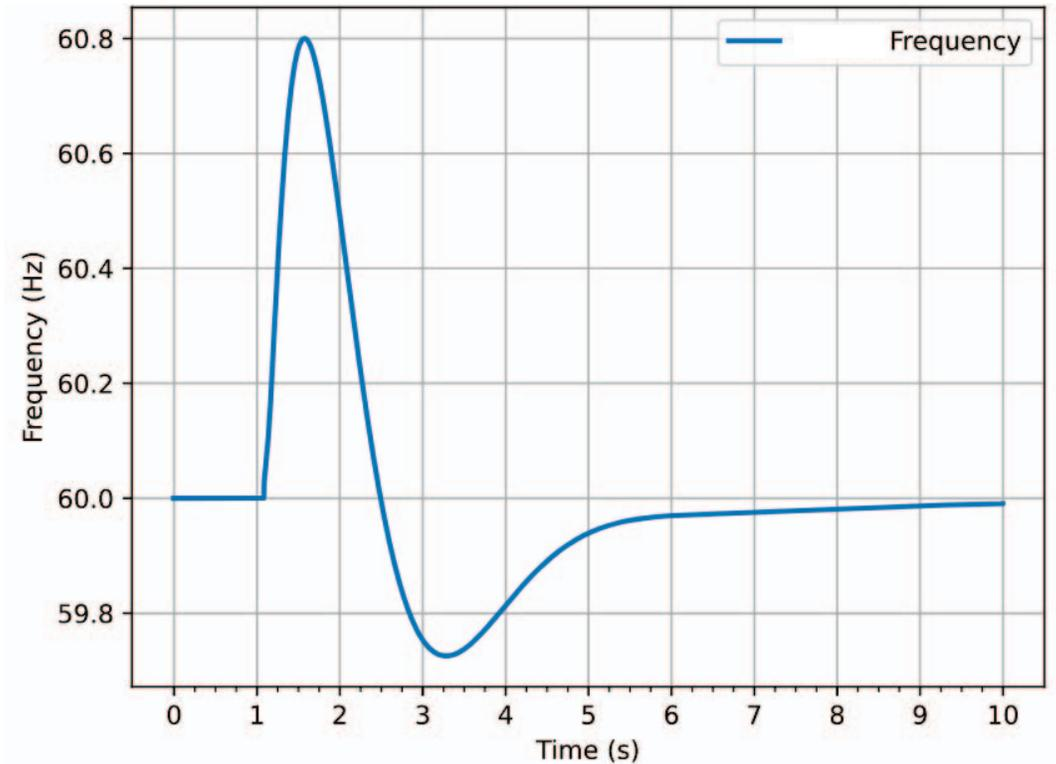
Fig. 11. Switchyard D East Bus Frequency for Island at Substation B 115 kV Bus with 2 Units Online (Winter)
