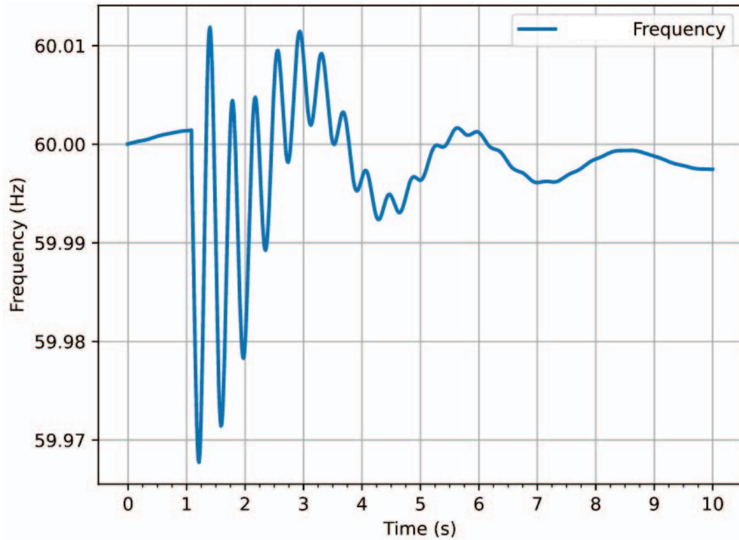
Fig. 5. Switchyard D West Bus Frequency for Island at Substation C 115 kV Bus with 4 Units Online (Summer)
