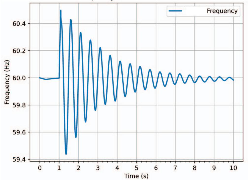
Fig. 17. Switchyard D West Bus Frequency for Fault at Substation B T3 with all Units in Service (Winter)
