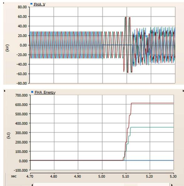
Fig. 4. Arrester Energy Waveform for 24.4kV MCOV
