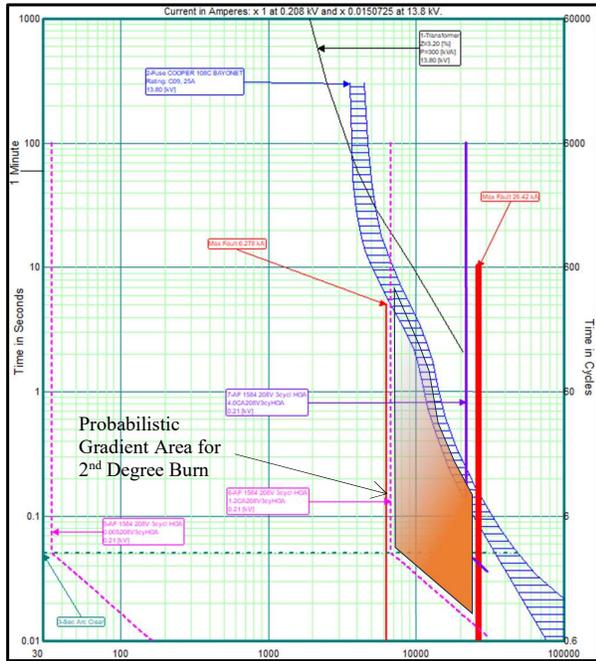
Fig. 6. Addition to Figure 5 the probabilistic gradient for second-degree burn for an arc flash progressing to a minor arc blast.
