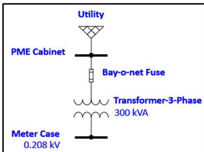
Fig. 3. One-line from the utility to a meter case.
