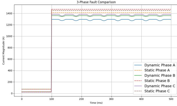
Fig. 8. Three Phase Fault Current Comparison for 25% BTM PV Penetration
