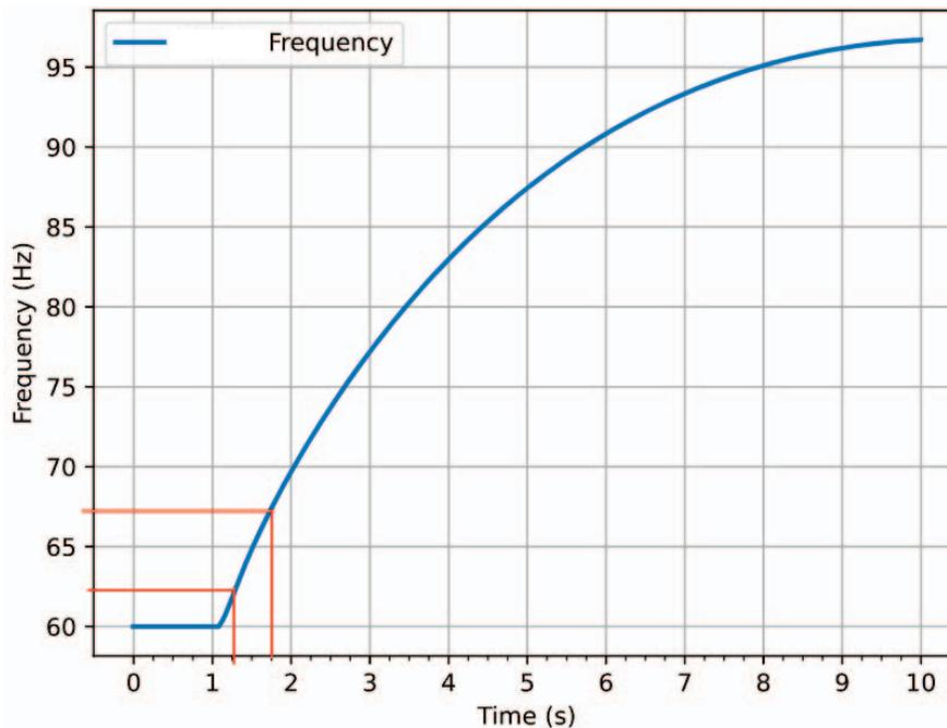
Fig. 4. Switchyard D West Bus Frequency for Island at Substation C – Substation A with 4 Units Online (Summer)
