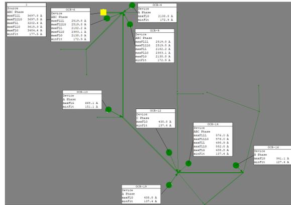
IMAGE 2: Arc flash calculations using the base point 7.5 MVA transformer.
