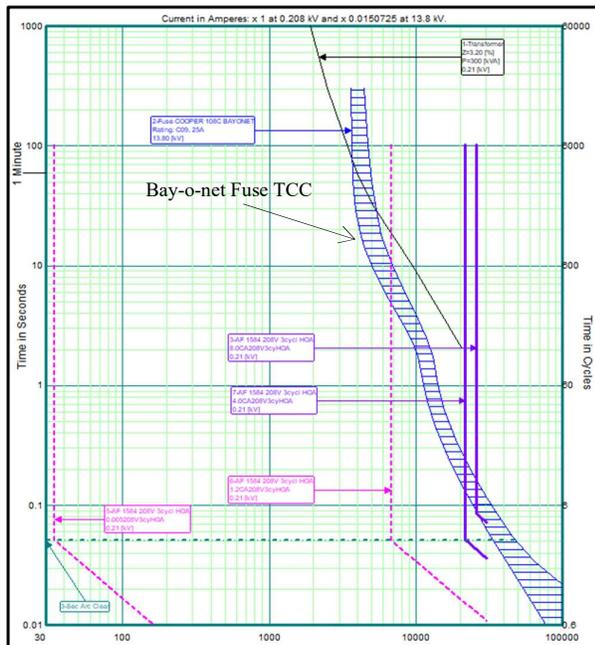
Fig. 4. Addition to Figure 1 a 300kVA transformer with a 25A fuse.
