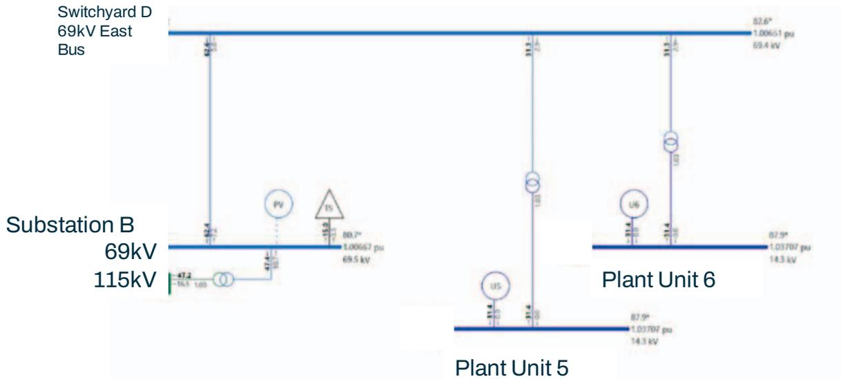
Fig. 3. WECC 2025 Light Winter Model of Switchyard D – Loop B – East Bus
