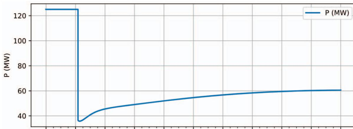
Fig. 6. Switchyard D West Bus Power Output for Island at Substation C 115 kV Bus with 4 Units Online (Summer)
