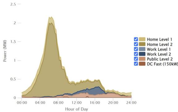
Fig. 2. Sample EV charging profile, Home: delayed-finish by departure, work: delayed-finish by departure.
