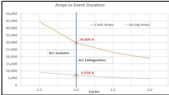
Fig. 2. Example plot of the calculated current levels of a 208V HOA event where the arc would exist and be extinguished.
