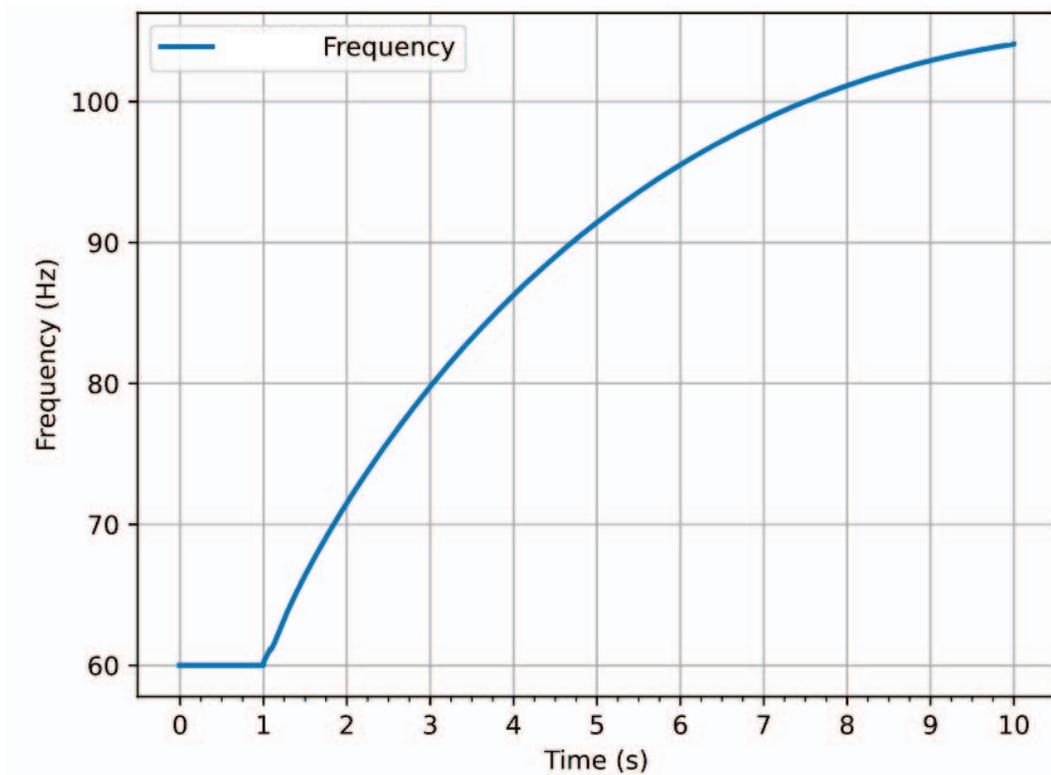
Fig. 15. Switchyard D East Bus Frequency for Fault at Substation B T3 with all Units Online (Winter)
