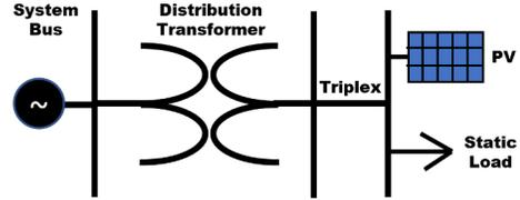
Fig. 4. Simple Composite Load Model with PV
