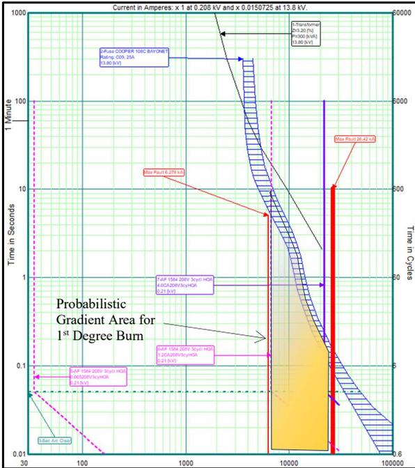
Fig. 7. Addition to Figure 5 the probabilistic gradient for a first-degree burn for an arc flash progressing to a minor arc blast.
