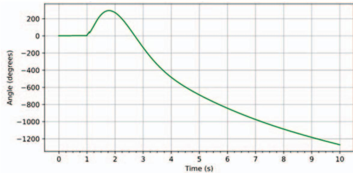
Fig. 9. Voltage Angle Difference Between Switchyard D and Substation E During an Island at Substation C T3 with 1 Unit in Service
