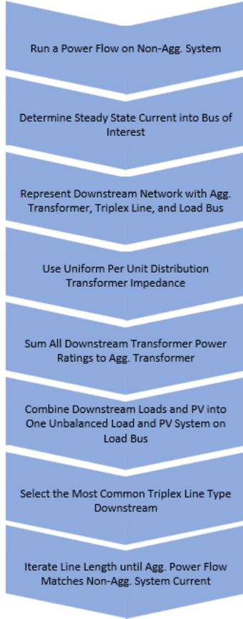
Fig. 6. Flow Chart of Simple Aggregation Method
