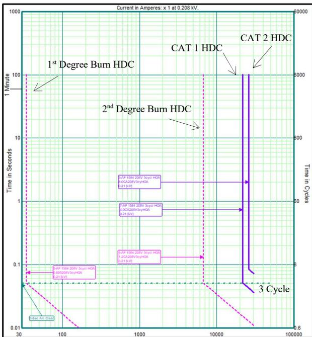
Fig. 1. HDC TCCs for first- & second-degree burn and PPE coverage for CAT 1 & 2.
